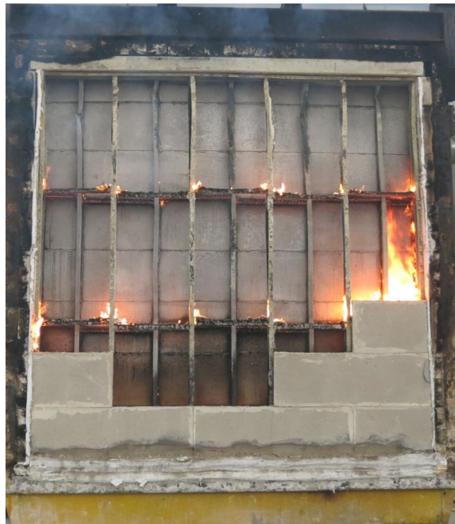
Figure A6.4 Exposed face of specimen at the end of the test
