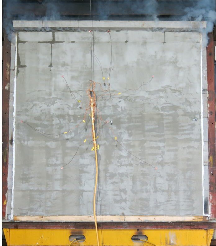
Figure A6.3. Unexposed face of specimen at the end of the test
