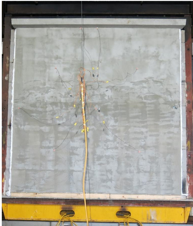
Figure A6.1. Unexposed face of specimen before commencement of the fire-resistance test
