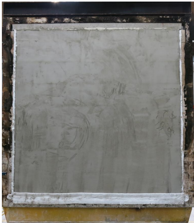
Figure A6.2. Exposed face of specimen before commencement of the fire-resistance test
